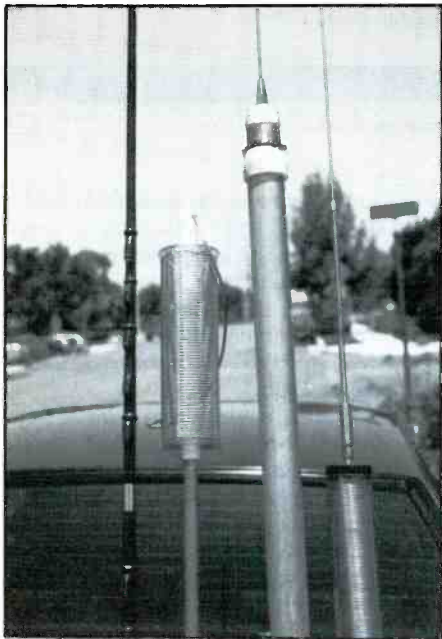
An HF whip for each band of operation will insure solid contacts from the command center.
