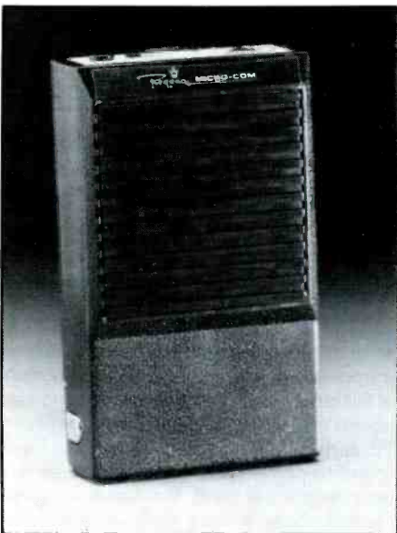
The Regency Micro-Com beeper is a modern paging receiver covering 148 to 160 MHz.
