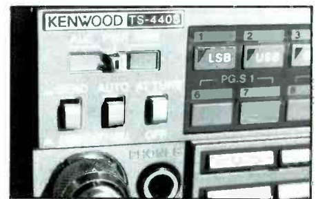
This auto-tuner built into the TS-440 will do a good job into a 50 ohm load.
